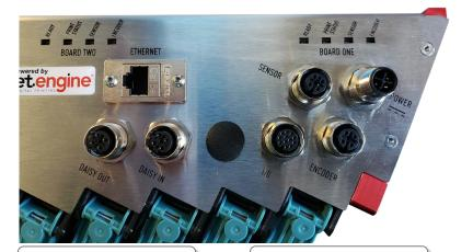
M12 Electrical Connections for Sensor, Encoder, Daisy Chain, and I/O Signals Mounting Points
